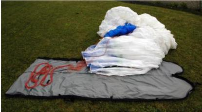
Sit on the opposite side of the bag and pull the cells onto the bag, one by one, from the nearest stable, across the middle and to the furthest stable.
