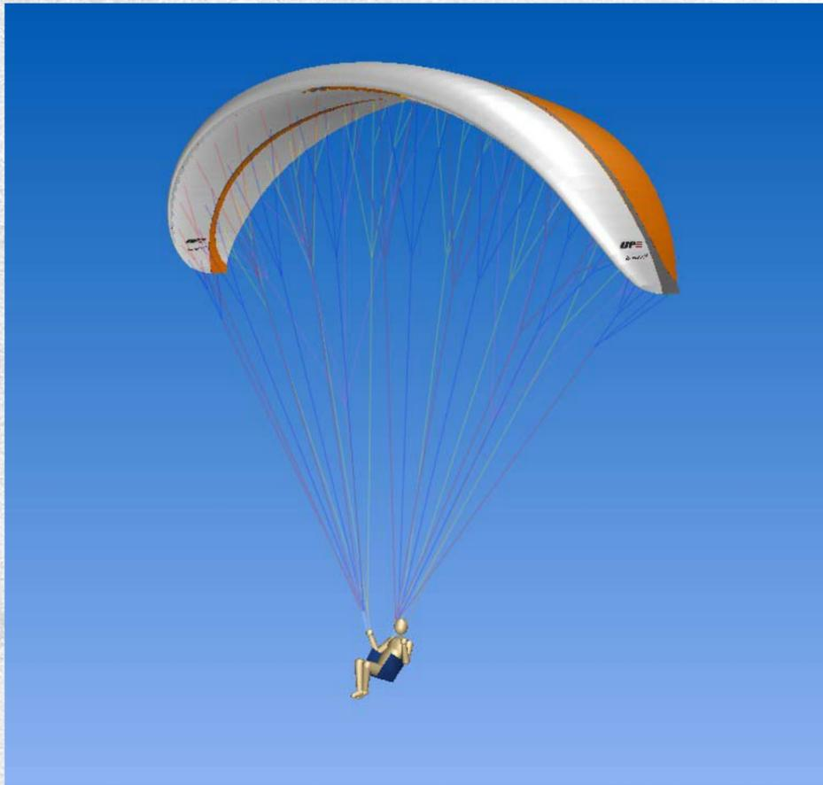
The 3-liner design in accordance with the swept back wingtips, first introduced in our comp wing protos and the Trango XC improve performance by reducing drag
