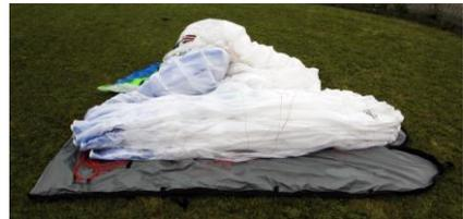
Also note that the leading edge ideally isn't stacked all at the top of the bag; rather, the gathered cells are "stepped" (see illustration) so that the short wingtip ones are in the middle of the pack, and the longer centre cells are the only ones that reach the very top of the bag.
