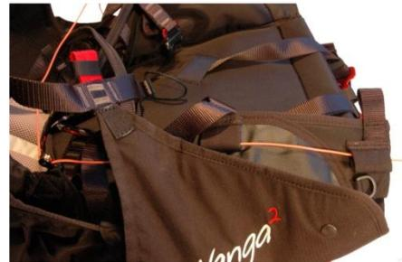
Start by threading the speedbar lines through the cloth loops on either side of the seat board. Then through the pulley and up to the brummel hooks on the risers.
