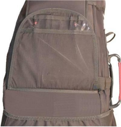
Place the reserve handle on the Velcro patch and stick both ends into the pockets at either end. The connection tape that runs to the inner container should be routed behind the webbing so that nothing may get caught on launch, causing an unintentional deployment.
