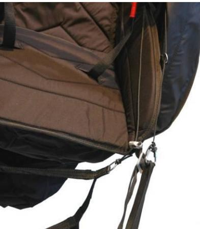
On the left hand side the line goes first through the metal pulley, then the grommet in the leg cover and then it is tied onto the plastic buckle.
