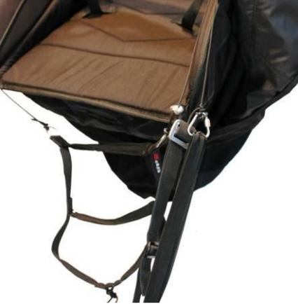
On the right hand side (flight direction) the closure line should be routed through the metal pulley and then tied directly onto the plastic buckle.
