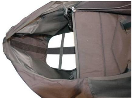
Now thread the stirrup strap through the buckle (remember to thread it through once more to lock it). Once adjusted the stirrup should be under light tension while in flying position.
