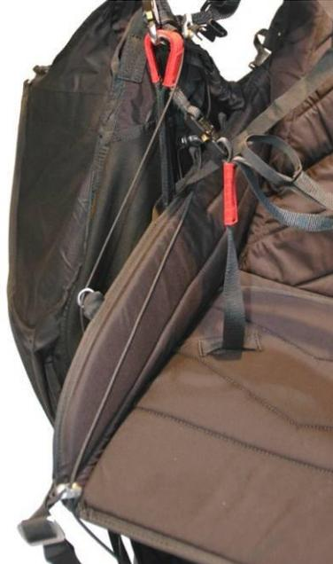
Attach the speed bar with the rubber bridle to the foot plate.
