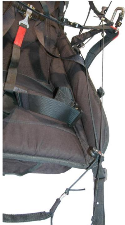
On the right hand side the closure line should be routed through the metal pulley and then tied directly onto the plastic buckle.
