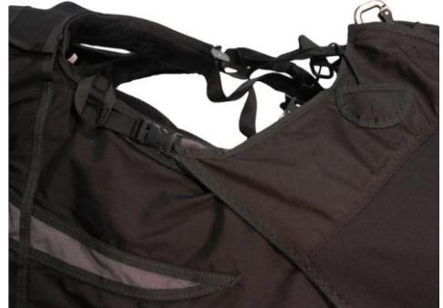
Open the neoprene covers on the shoulders. Inside you'll find a plastic buckle that is used for attaching the long elastic band from the leg cover. In flight the elastic band should only be just tensioned as any more tension carries the risk of overstretching the elastic.
