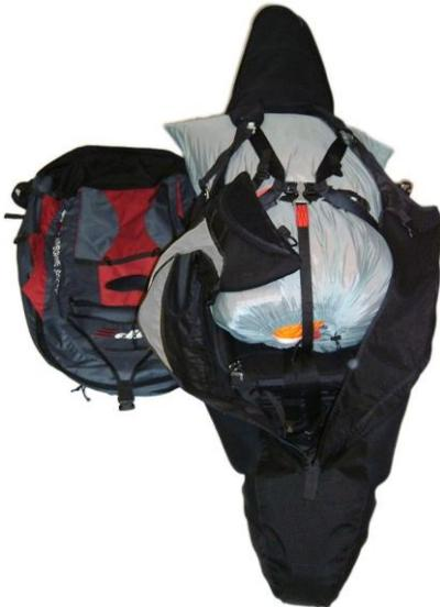
**BEWARE!** The back cone contains a variety of reinforcements, all serving to maintain the aerodynamic shape in flight. To prevent excessive buckling of these the rear compartment should be opened for packing, and the lid routed over the packed wing.
