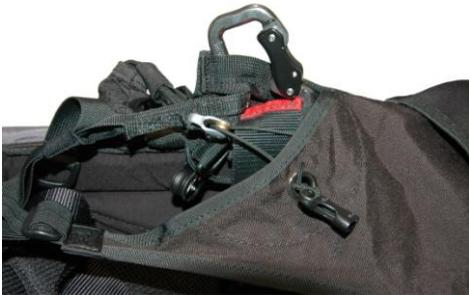
Adjust the bungee so that the foam nose cone of the leg cover does not touch the ground during the launching phase. At the same time, make sure the closure lines are adjusted so that the harness is closed cleanly when the flying position has been reached in flight.
