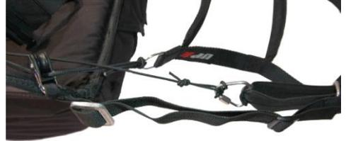
The foot plate bungee strap goes through the metal hoops for the stirrup and connect to the leg cover skirt closing line using the Delta-Maillon. The closing line is then routed through the lateral metal rings to the little pulleys on the shoulder straps.
